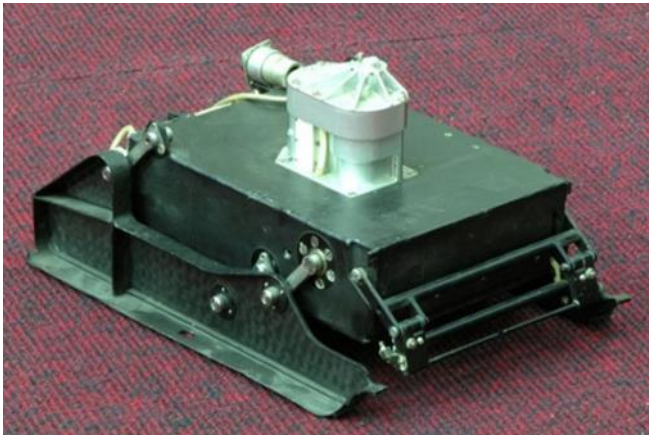
Figure 1. Mars Prop-M (Passability Assessment Device)
